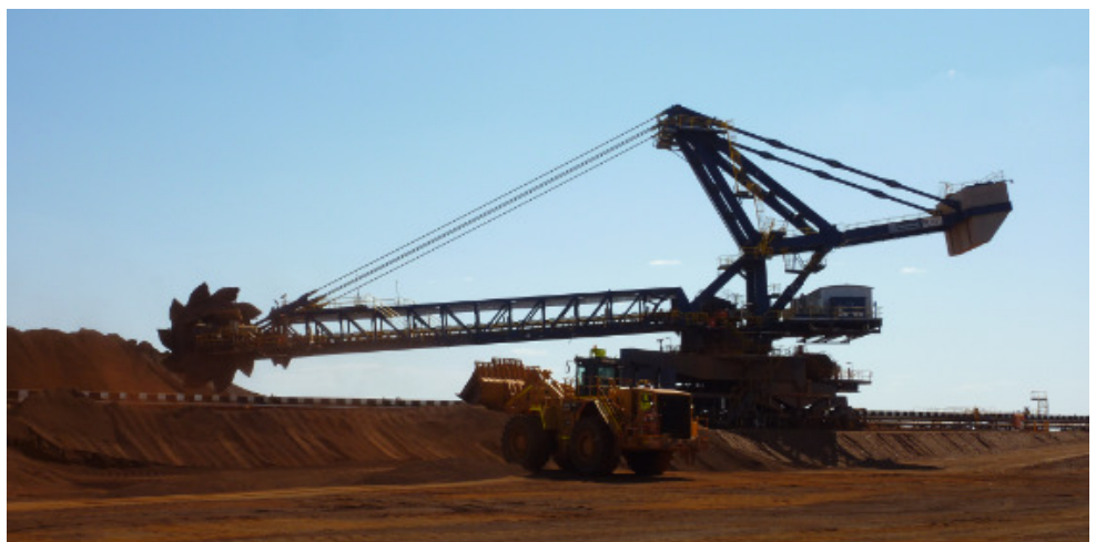
Figure 6: FMG’s Load-Out Reclaimer at Christmas Creek
