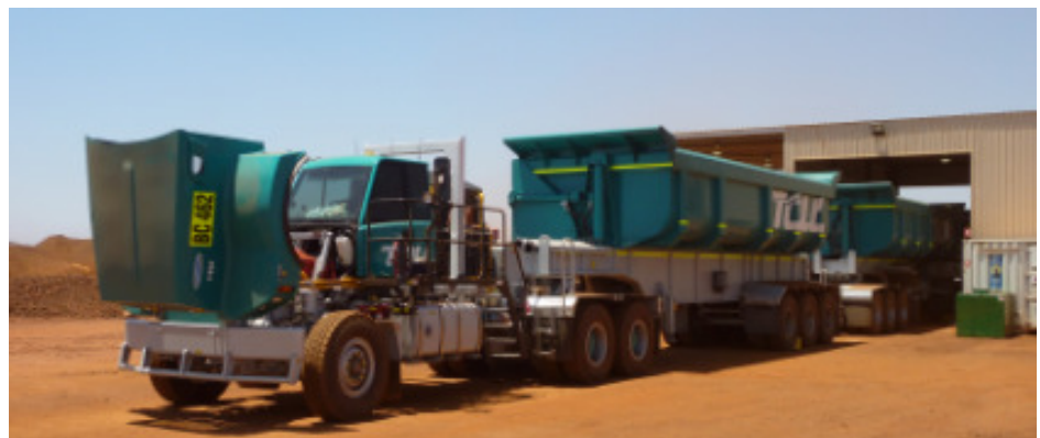
Figure 4: 360t Pit Haulers (now commissioned)
